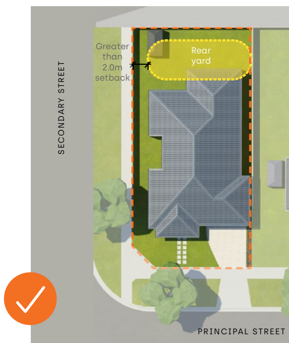
Outbuilding located in rear yard. Setback 2m from side boundary for corner lots, addressing a secondary street.
