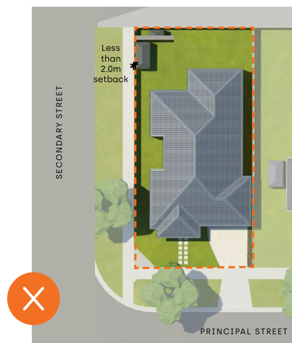
Outbuilding located to side of dwelling and visible from primary street address
