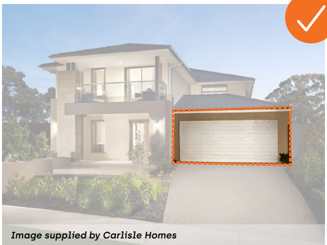
DIAGRAM 09 - GARAGES TO BE SETBACK A MINIMUM OF 5.0M FROM THE PRINCIPAL STREET FRONTAGE TO ALLOW FOR PARKING OF ONE VEHICLE
