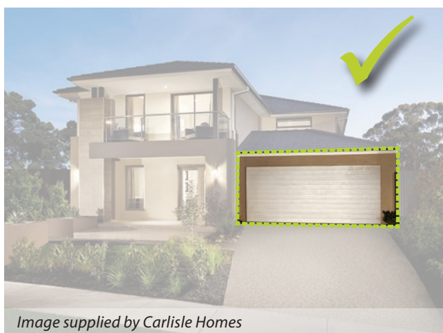
Diagram 08 - Garages to be setback a minimum of 5.0m from the principal street frontage to allow for parking of one vehicle
