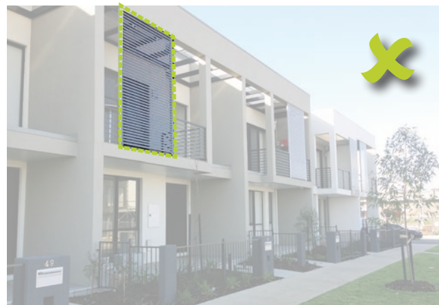
Diagram 12 - Window screening located on the primary frontage will not be approved.
